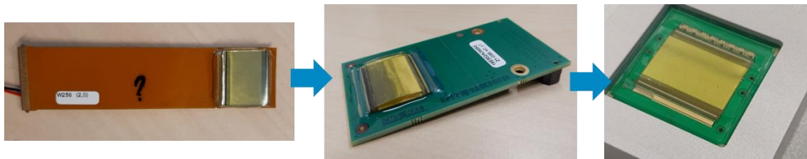
Figure 17: Three versions of assembled CMUT modules. Left: version A with CM5 and acoustic stack mounted on flex. Middle: version B, same acoustic stack mounted on PCB. Right: version C with improved assembly method and acoustic stack with PCB mounted in metal housing
